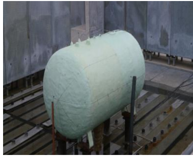
Figure 6. 2,75m 3 Storage tank with fire protection coating before the test (example)
