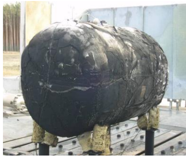
Figure 7. 2,75m 3 Storage tank with fire protection coating after the test
