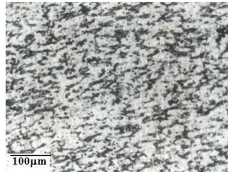
Figure 6. Optical micrograph of 75% cold rolled alloy 3.
