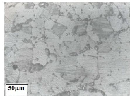
Figure 7. Optical micrograph of 75% cold rolled alloy 1, annealed at 400 °C for 1 hour.
