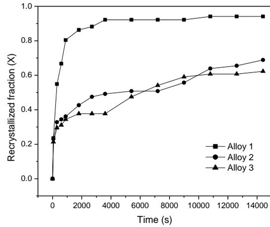
Figure 2. Recrystallization kinetics obtained from microhardness data.
