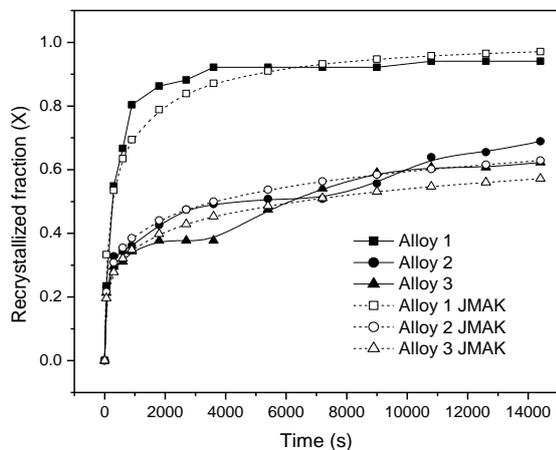
Figure 4. Recrystallization kinetics for the alloys from Micro-hardness data and JMAK analysis.
