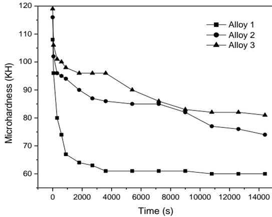
Figure 1. Isothermal annealing curve of the alloys, annealed at 400 °C.
