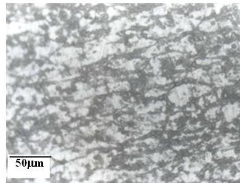
Figure 8. Optical micrograph of 75% cold rolled alloy 3, annealed at 400 °C for 1 hour.
