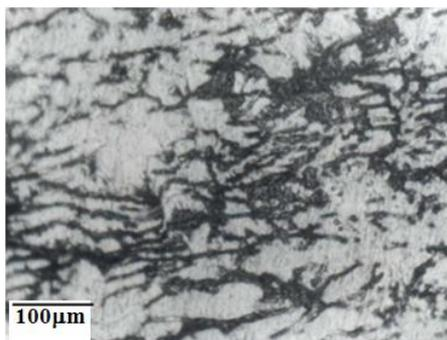
Figure 5. Optical micrograph of 75% cold rolled alloy 1.
