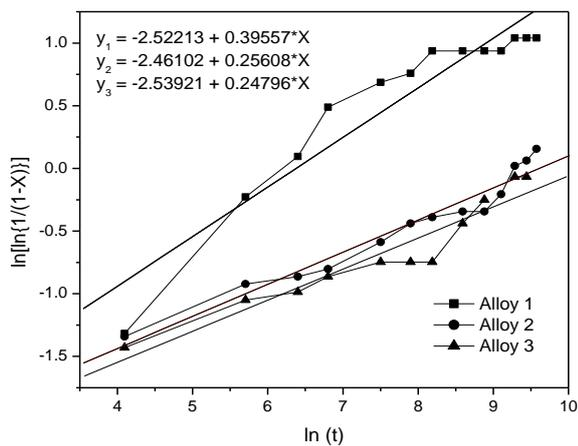
Figure 3. Plot of  $\ln[\ln\{1/(1-X)\}]$  Vs.  $\ln(t)$ , showing a linear relationship with a slope equal to the JMAK exponent.
