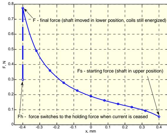
Figure 6. Force-stroke characteristic of the optimal actuator. Coils are energized. The shaft is displaced from final upper to final lower position.
