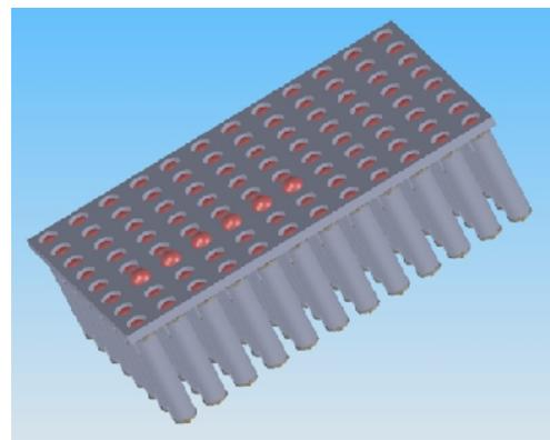
Figure 9. A 3D CAD model of the Braille screen.
