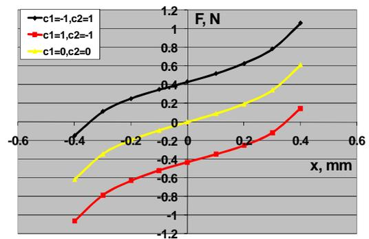
Figure 4. Force-stroke characteristics for  $h_m=2$  (mm),  $\delta=3$ (mm),  $h_w=5$  (mm),  $I_w=180$  (A),  $J=20$ (A/mm<sup>2</sup>).
