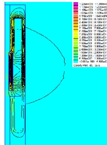
Figure 8. Magnetic field of the optimal actuator with no current in the coils.
