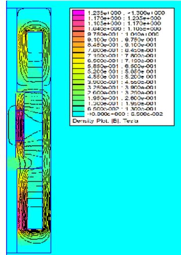
Figure 7. Magnetic field of the optimal actuator with shaft in upper position and energized coils.
