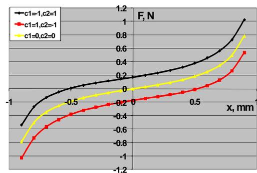
Figure 5. Force-stroke characteristics for  $h_m=2$  (mm),  $\delta=5$  (mm),  $h_w=10$  (mm),  $I_w=180$  (A),  $J=10$  (A/mm<sup>2</sup>).
