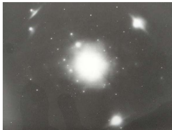
Fig. 15. SAD pattern of the matrix and the precipitates of alloy 3 aged at 300°C for 1 hour.
