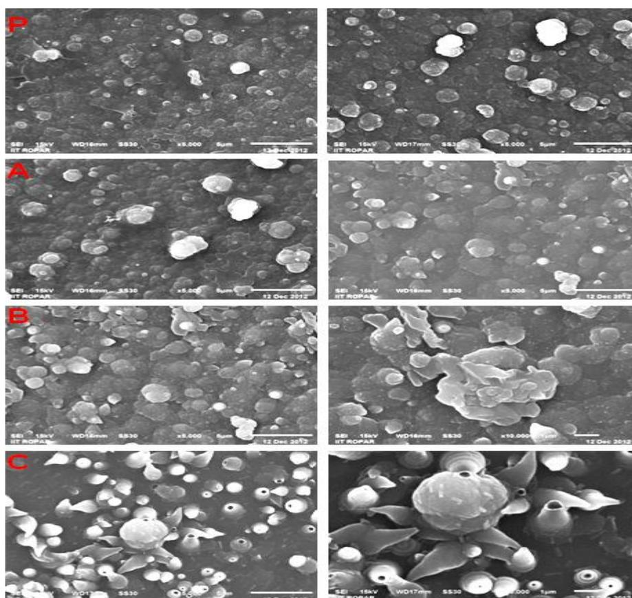
Fig. 2. SEM images of pristine and Ni<sup>9+</sup> ion irradiated Ag-PPy composite films at (A)  $3 \times 10^{11}$  ions/cm<sup>2</sup>, (B)  $1 \times 10^{12}$  ions/cm<sup>2</sup>, and (C)  $3 \times 10^{12}$  ions/cm<sup>2</sup> with their magnified images.
