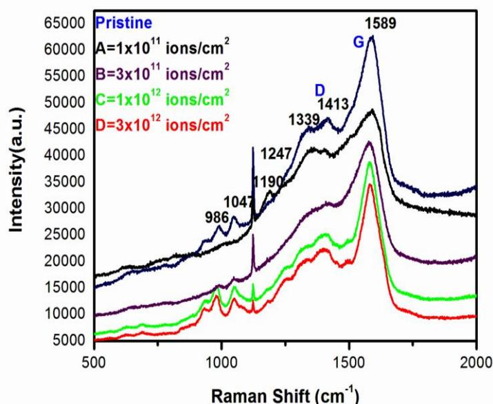
Fig. 1. Raman spectra of pristine and irradiated Ag-PPy composite film irradiated with 120 MeV  $Ni^{9+}$  at various fluences.
