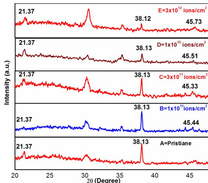
Fig. 3. XRD spectra of pristine and 120 MeV  $Ni^{9+}$  ion irradiated Ag-PPy film at different fluences (B) =  $1 \times 10^{11}$  ions/cm<sup>2</sup>, (C) =  $3 \times 10^{11}$  ions/cm<sup>2</sup>, (D) =  $1 \times 10^{12}$  ions/cm<sup>2</sup> and (E) =  $3 \times 10^{12}$  ions/cm<sup>2</sup>.
