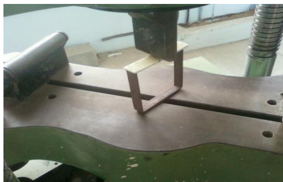
Fig. 3. Mode II Inter laminar fracture toughness test
