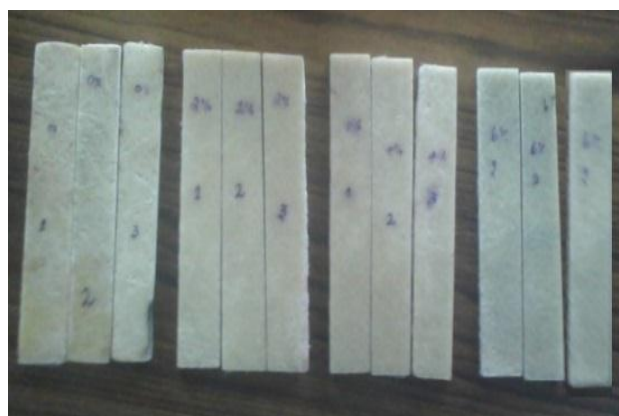
Fig. 1. Fabricated ENF Test specimens
