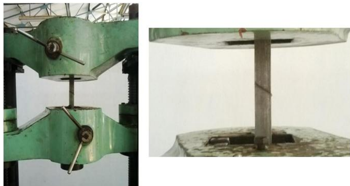
Fig.4. Testing of scarf adhesive joint on UTM
