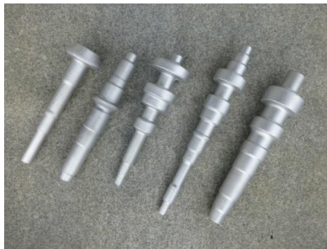
Fig. 3. SMART forged products before gear cutting process.
