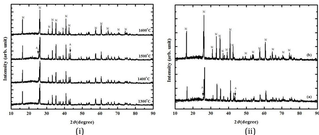
Fig.1. XRD pattern of silica xerogel loaded by 60 wt%  $\alpha$ -Al $_2$ O $_3$  and sintered at (i) different temperature and (ii) 1600°C by (a) conventional heating [6], and (b) microwave heating of a 28 GHz gyrotron.
