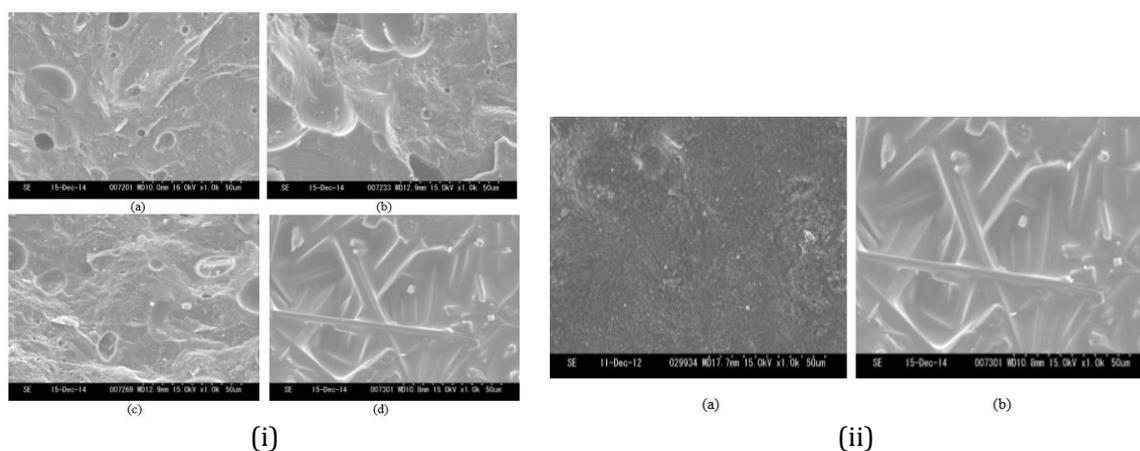
Fig. 2. SEM images of silica xerogel loaded by 60 wt%  $\alpha$ -Al<sub>2</sub>O<sub>3</sub> and (i) sintered at (a) 1300°C, (b) 1400°C, (c) 1500°C, and (d) 1600°C, and (ii) 1600°C by (a) conventional heating [6], and (b) microwave heating of a 28 GHz gyrotron.
