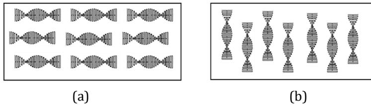
Fig. 2. (a) Focal conic texture and (b) planar texture [2].
