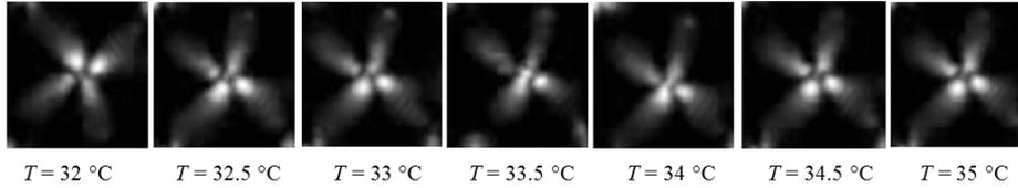
Fig. 6. Crossed-twist pattern images at over higher critical temperature of TLCs sample.
