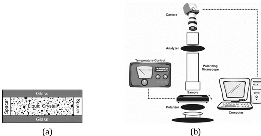
Fig. 5. (a) Side view of sample. (b) Instrumentation set-up.
