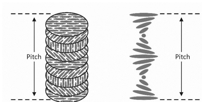
Fig. 1. Molecules alignment of chiral nematic liquid crystal structure.
