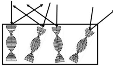
Fig. 4. Bragg scattering illustration of non-normal incident light in chiral nematic.
