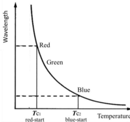
Fig. 3. Graph of reflected wavelengths at various temperatures. Critical temperature notated by  $T_c$  representing red-start at lower temperature  $T_{c1}$  and blue start at higher temperature  $T_{c2}$  [2].
