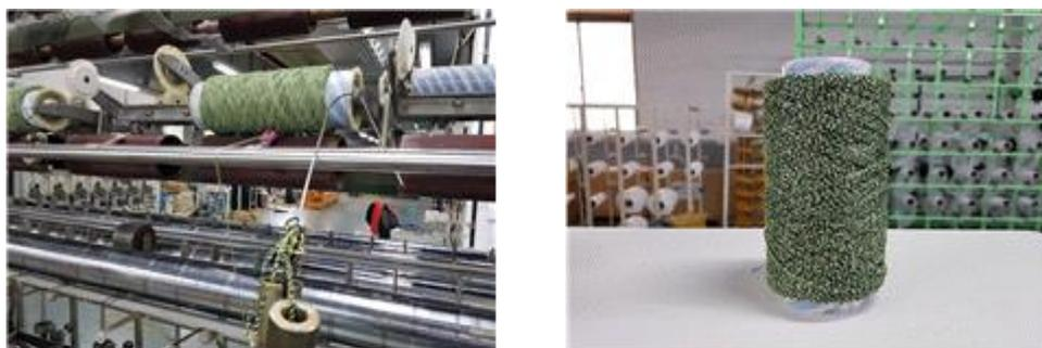
Fig. 2. Carbon fiber composite yarn for grid fabric manufacturing.
