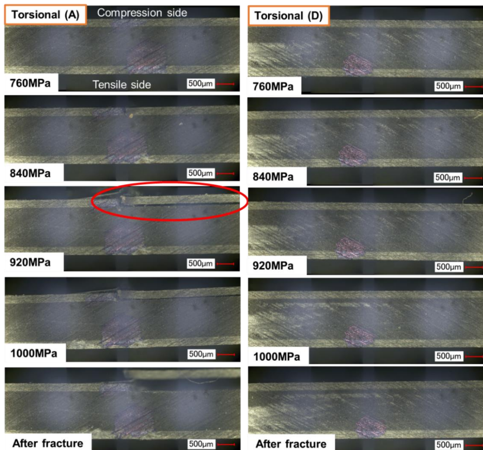
Fig. 6. Typical observation results of [0/30_s/0] laminates under “Torsional” condition.
