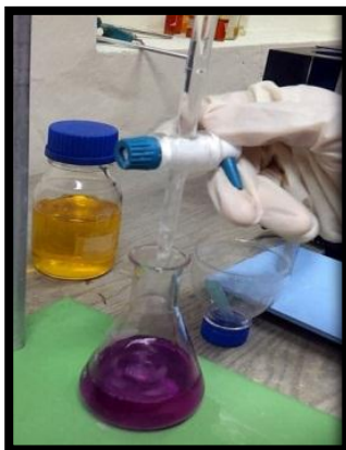
Figure 10. Purple color is indicator to show the acid number
