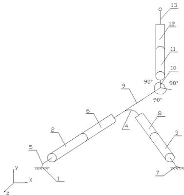
Figure 11. Micro manipulator with 3 DoF and incorporated electromagnetic actuators into its links.
