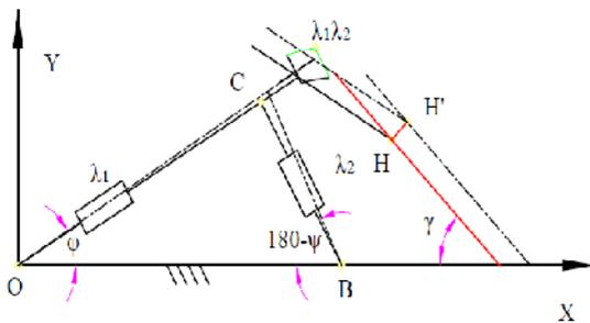
Figure 13. Structural scheme of 2 DoF mechanism with electromagnetic actuators.
