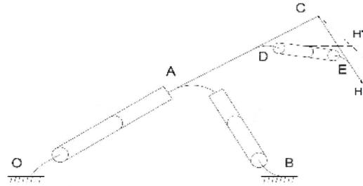
Figure 12. Structural scheme of 3 DoF mechanism with electromagnetic actuators.
