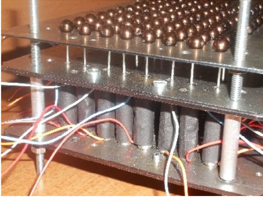
Figure 10. A prototype of Braille screen with needles (dots) driven by linear actuators.
