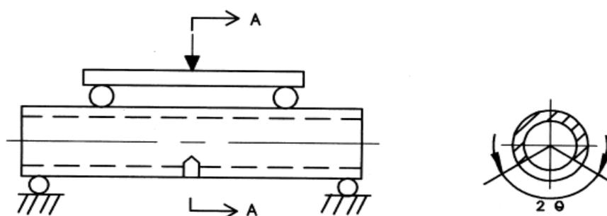
Fig. 6. Geometry of pipe specimen.[1]
