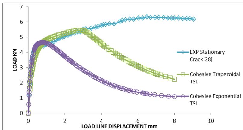
Fig. 5. Load vs load line displacement for TPB specimen
