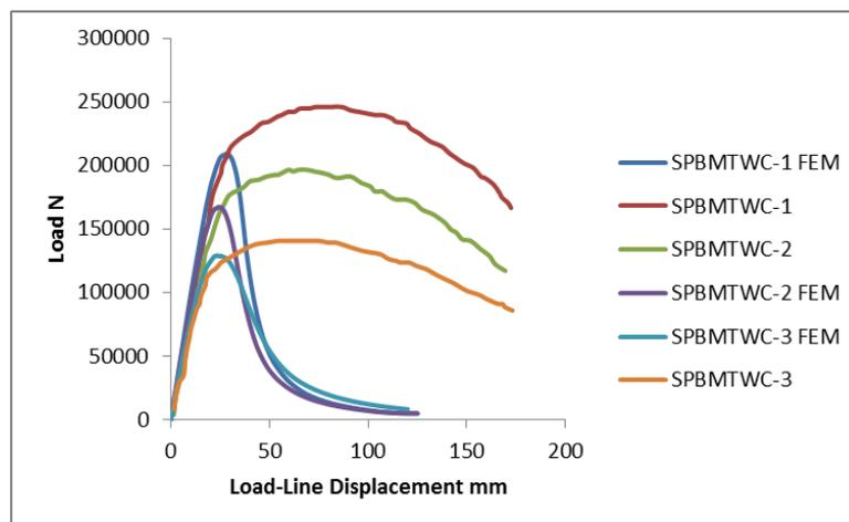
Fig. 9. Experimental load vs. load point displacement curves for pipes.
