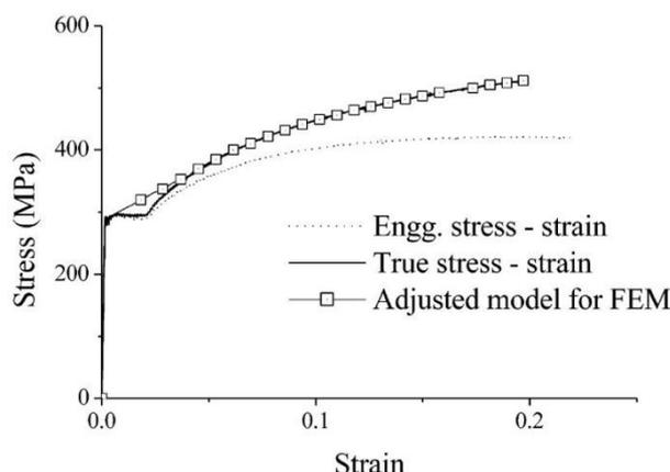
Fig. 1. Stress-strain diagram for tensile samples machined from 219 mm OD pipes [28]
