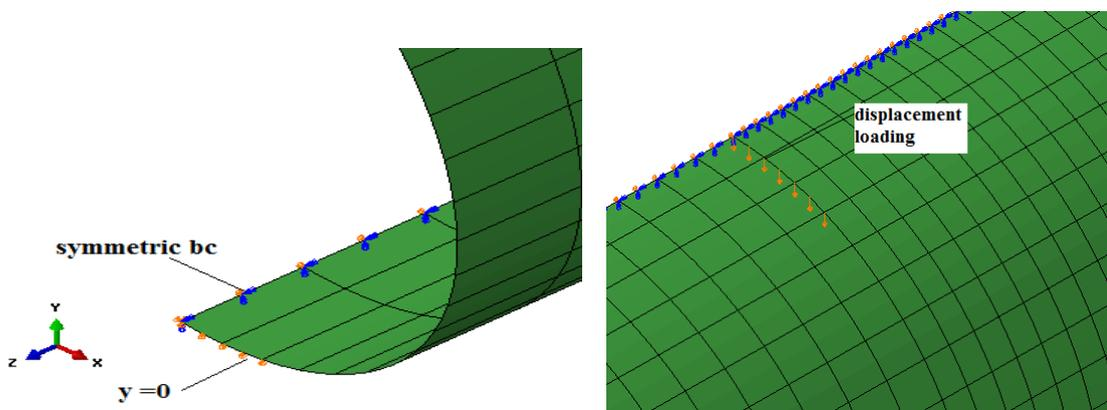
Fig. 8. Boundary condition on the pipe model
