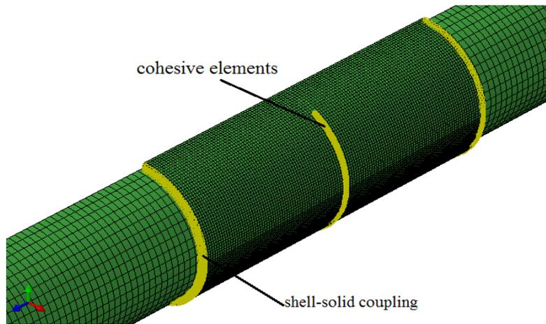
Fig. 7. Finite element mesh on pipe specimen SPBMTWC-1
