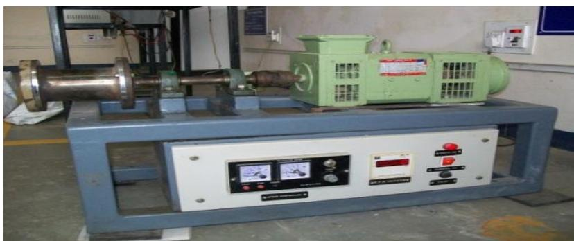
Fig. 1. Horizontal centrifugal casting machine.
