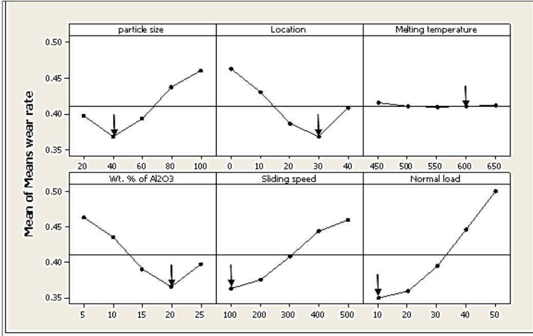
Fig. 2. Relative effect of main factors on wear rate of the ZA-27/Al<sub>2</sub>O<sub>3</sub> composites at sliding distance of 1 km
