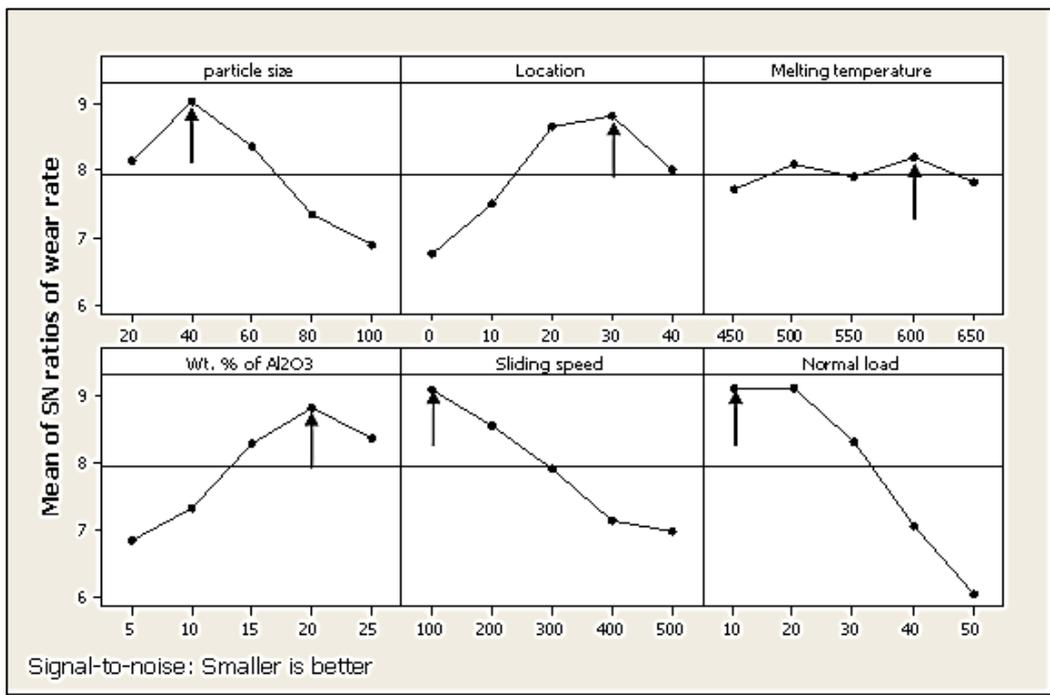
Fig. 3. Relative effect of S/N ratio on wear rate of the ZA-27/Al<sub>2</sub>O<sub>3</sub> composites at sliding distance of 1 km
