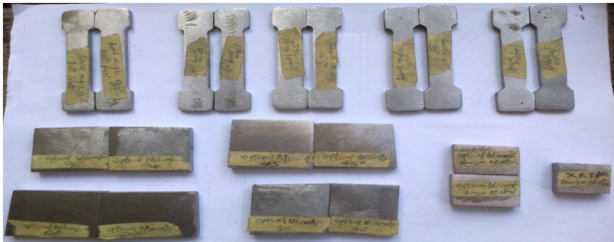
Fig. 2. Machined (milled) tensile and microstructures test samples
