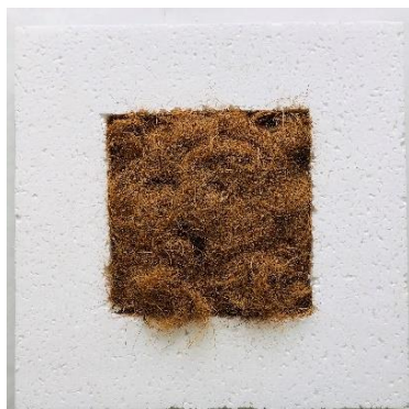
Fig. 1. Tested sample used for thermal conductivity test.
