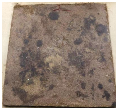
Fig. 2. Tested composite panel from coir fiber reinforced with PF resin used for thermal conductivity test (this figure was adapted under BN-CC 4 open access permission [17]).
